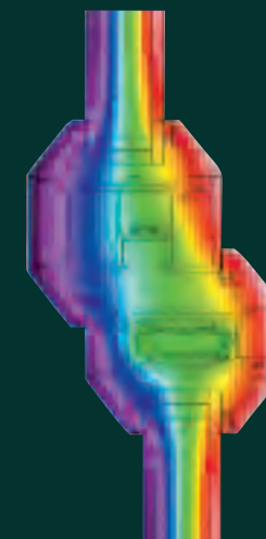
Thermal transfer through Liniar 'A Rated' sash/transom
